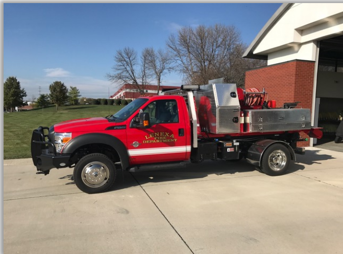
Utility 94 Equipped with a Brush Response Pod
